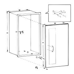
\*NOTE:These are rough openings for Fire-Rated Occult Series cabinets. Rough openings for non-rated rated cabinets are smaller - please refer to the appropriate non-rated Occult Series Submittal and Detail Sheet. Rough openings must be cut to the exact specifications or the fire rating will be void.
