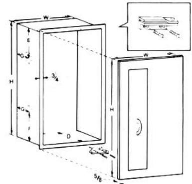
\*NOTE: THE ABOVE DIMENSIONS ARE FOR NON FIRE-RATED CABINETS, ROUGH OPENING DIMENSIONS AS WELL AS OUTSIDE FLANGE AND DOOR DIMENSIONS ARE LARGER FOR FIRE-RATED OCCULT CABINETS - SEE FIRE-RATED OCCULT SERIES.
