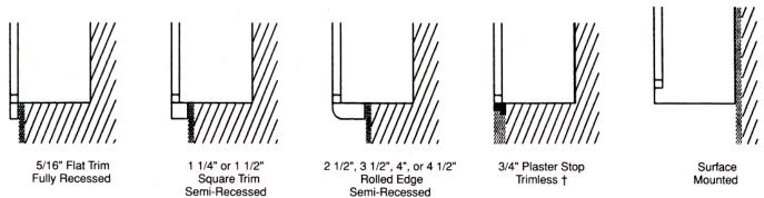
† Trimless cabinets must be installed before the drywall because their plaster stops must be behind the drywall. Trimless cabinets are not recommended for block wall installation.
