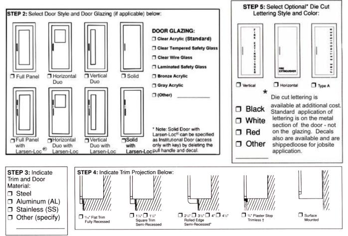
† Trimless cabinets must be installed before the drywall because their plaster stops must be behind the drywall.
